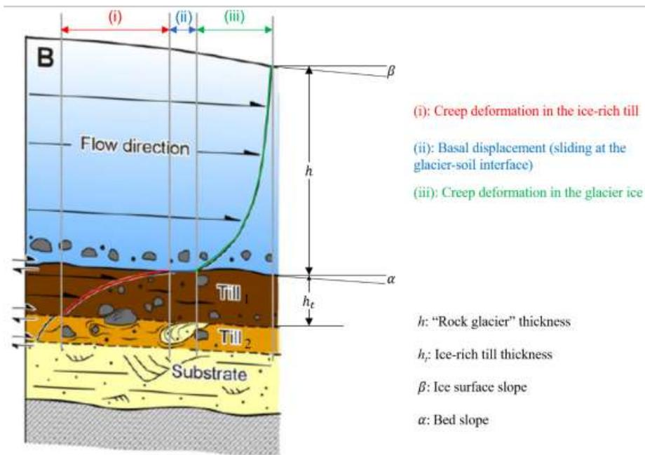
Figure 7. Displacement model. Deforming bed model graphic extracted from Ingólfsson et. al (2016) and further annotated.
