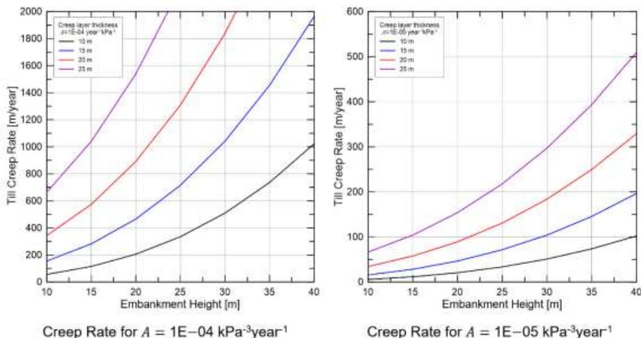
Figure 8. Glacial till creep rates as a function of creep parameter, till thickness and embankment height (rock loading).
