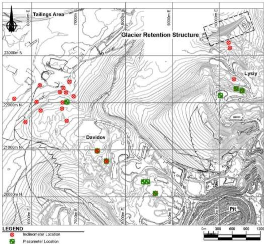
Figure 9. Glacier Retention Structure location and available inclinometer and piezometer data locations.
