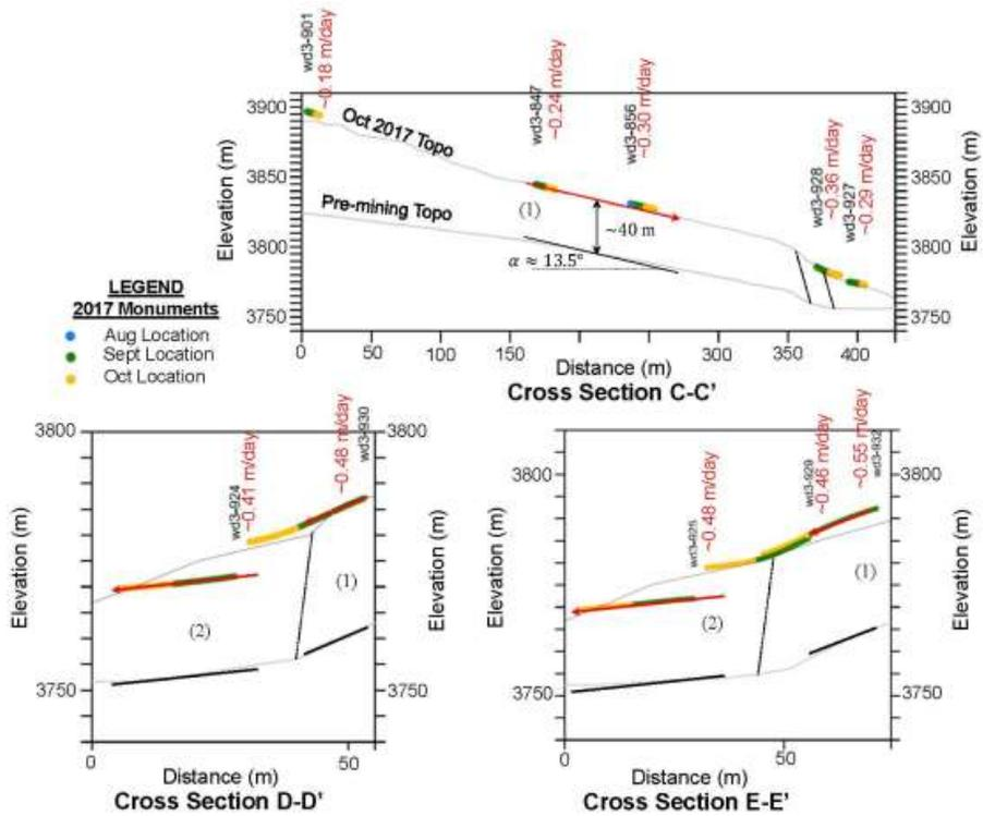
Figure 6. Movements of the NEV-WRD along section C, D and E.
