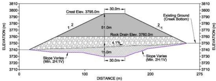
Figure 10. Typical cross sections through center of the conceptual Glacier Retention Structure
